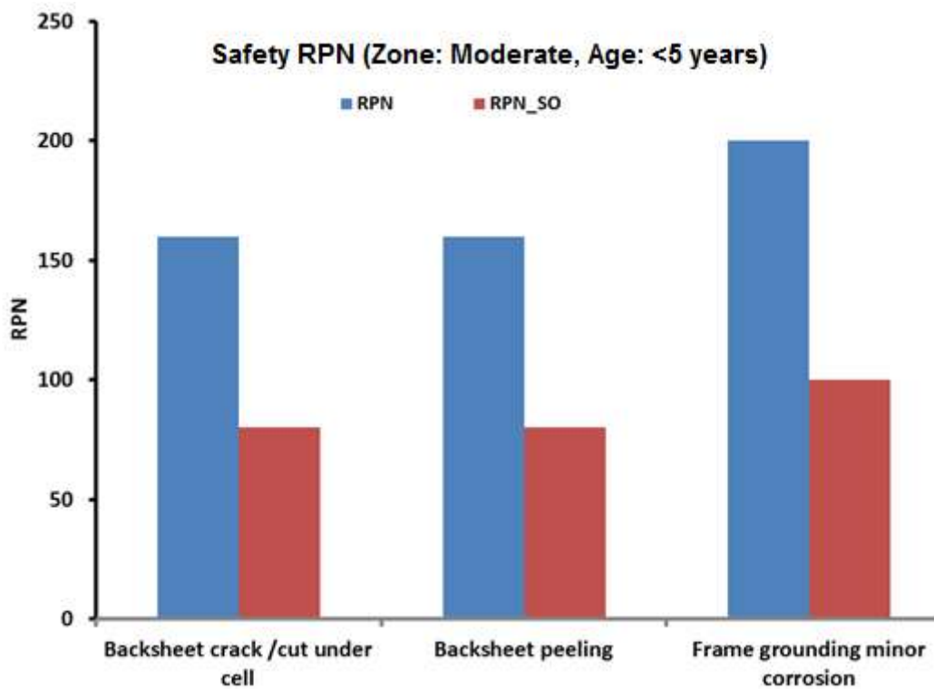
Fig. 8.13: RPN of different defects for Moderate zone for modules with less than 5 years of exposure – (a) Performance RPN, and (b) Safety RPN.
