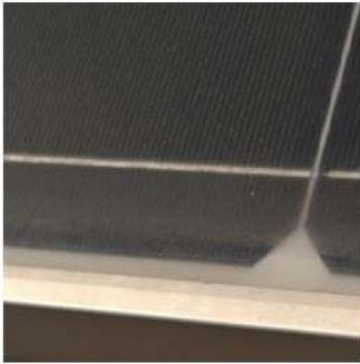
(a) Haziness in glass observed in old modules
