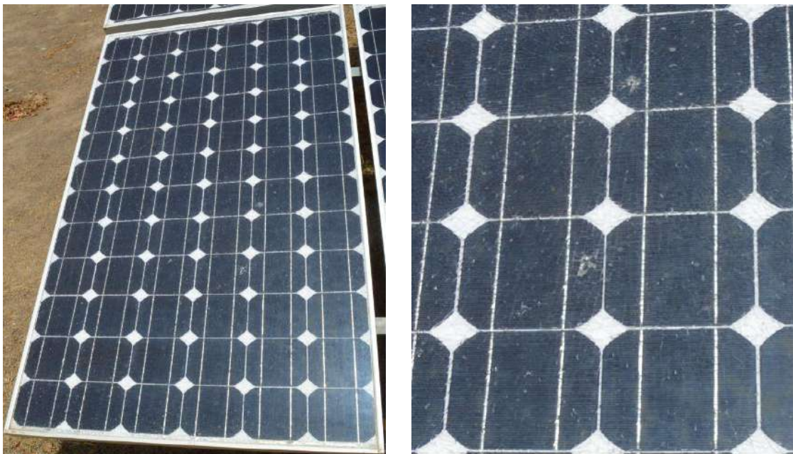
Fig. C.1. Visual Images of a Glass Broken PV Module
