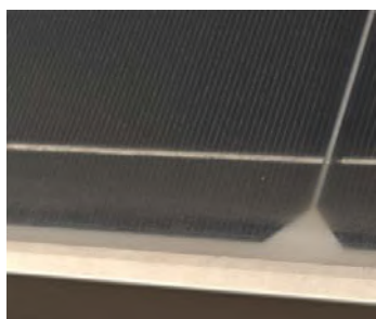
(a) Haziness in glass observed in old modules
