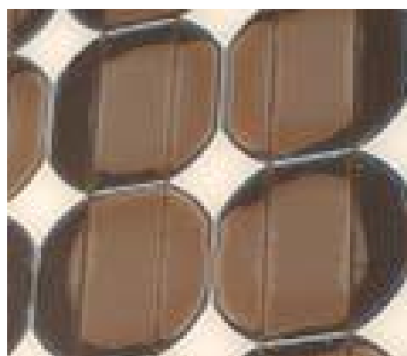
(b) Front-side delamination over cells in an old module in Warm & Humid zone (lighter in colour)
