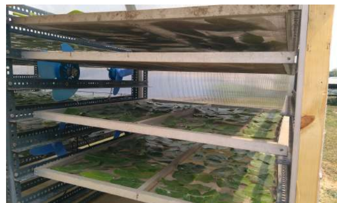
Figure 5.6 Greenhouse Dryer developed by NISE: (a) Lab scale prototype, (b) Lab testing
