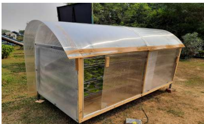
Figure 5.6 Greenhouse Dryer developed by NISE: (a) Lab scale prototype, (b) Lab testing
