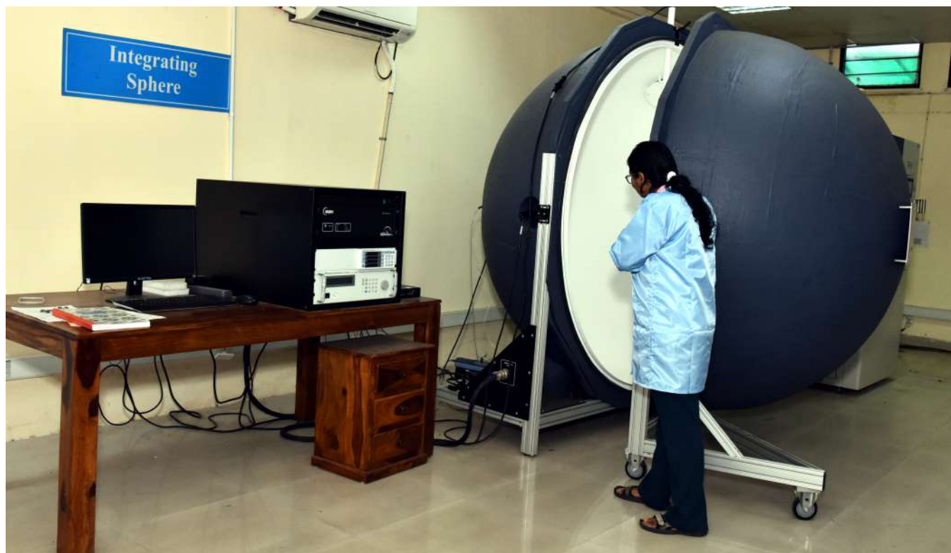
Figure 4.8 Integrating sphere system with temperature control for testing of solar street lights
