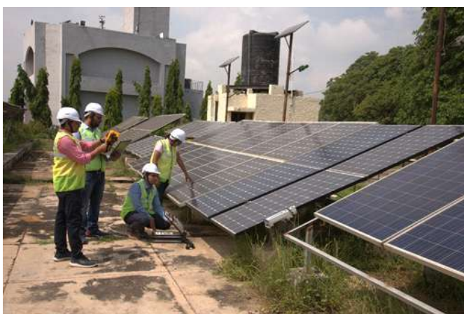
Figure 4.9 Testing of PV modules in test bed at NISE
