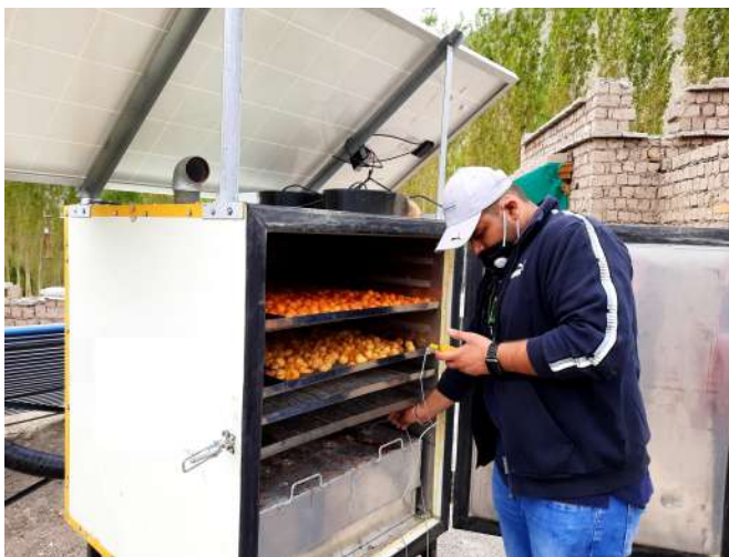
Figure 5.2 Solar Dryer-cum-Space Heating systems installed in Ladakh
