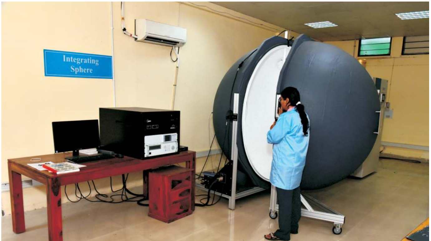
Figure 3.3: A photograph of luminaire testing facility with integrated sphere
