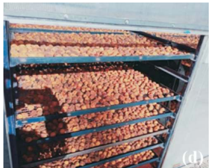
Figure 2.10: Mini-Greenhouse based Solar Dryer (a) Field testing in Ladakh, (b) Placing of apricots on mesh tray, (c) Fresh apricots fed inside the dryer, (d) Apricots during the drying process
