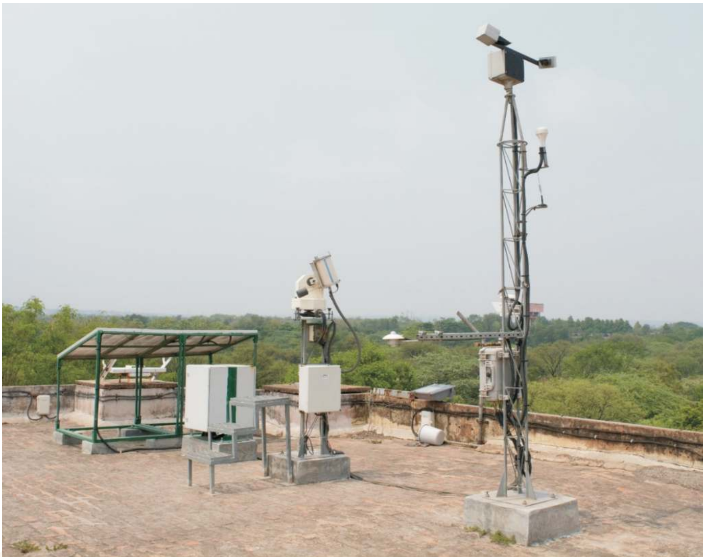
Figure 3.8: Solar Radiation Resource Assessment (SRRA) station facility at NISE.
