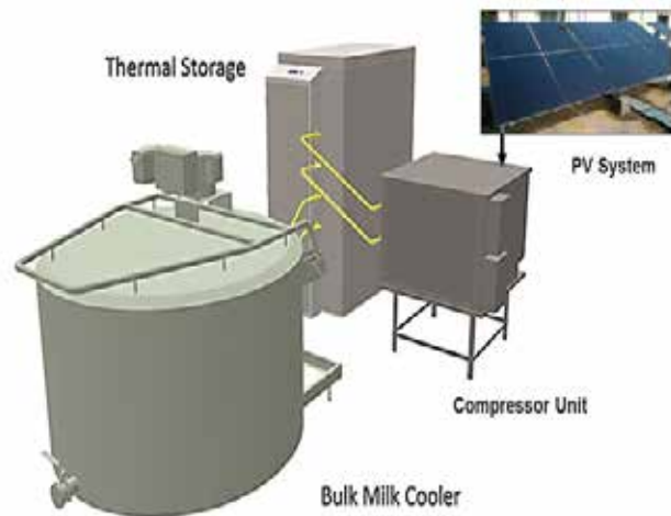
Solar Photovoltaic Bulk Milk Cooler using Thermal Storage
