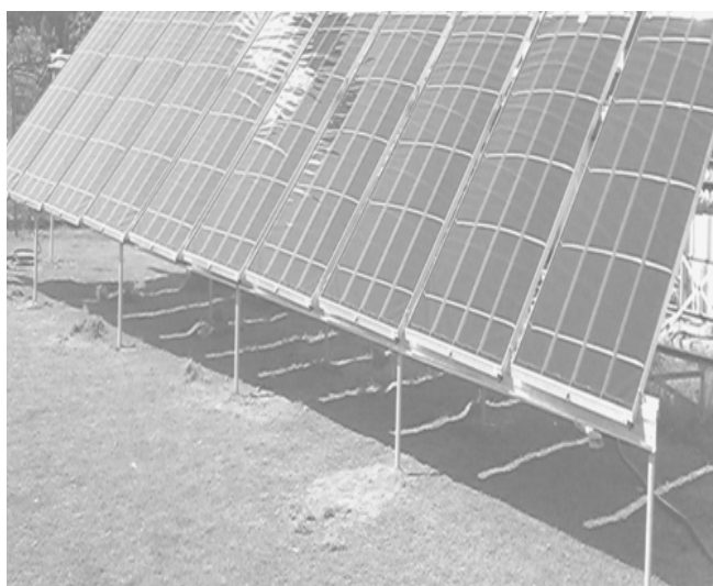
Experimental setup of Flat Plate type Solar Water Distillation system
