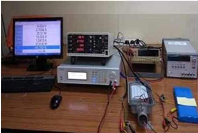
Driver Efficiency, Performance & protection testing of Charge Controller/Solar Inverter
