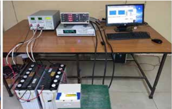
Driver Efficiency, Performance & protection testing of Charge Controller/Solar Inverter
