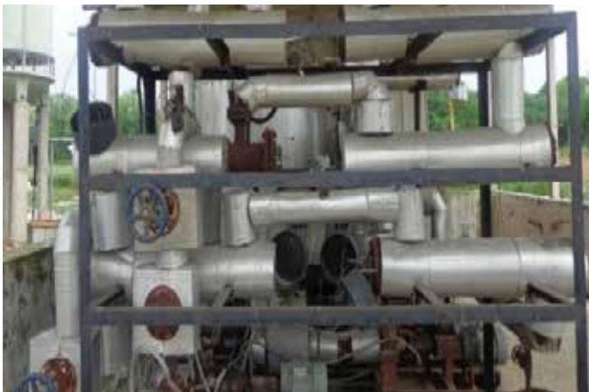
Thermic fluid based Test Set-up for CSTs at NISE
