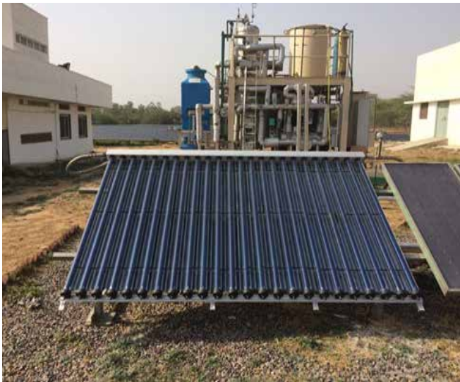
Test facility for testing of hot water/steam based CST systems
