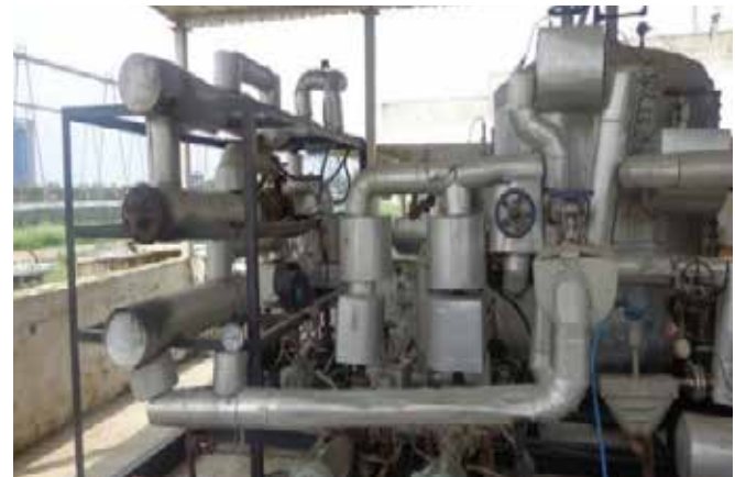
Thermic fluid based Test Set-up for CSTs at NISE
