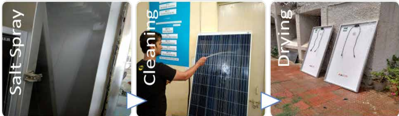
Pictorial representation of Salt spray test Sequence.
