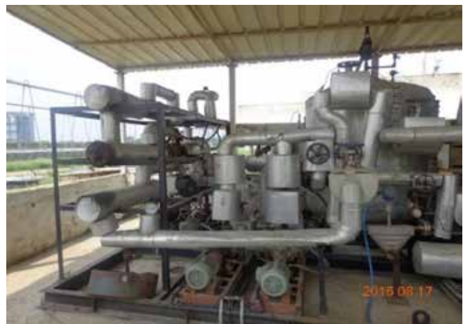
Figure 5.12 : Thermic fluid-based Test Set-up for CSTs at NISE
