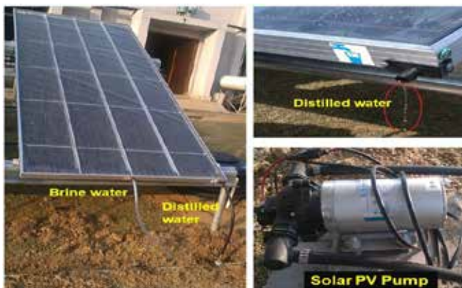
Figure 5.8: Experimental setup of Flat Plate type Solar Water Distillation system
