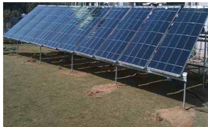
Figure 5.9: Experimental setup of Flat Plate type Solar Water Distillation system
