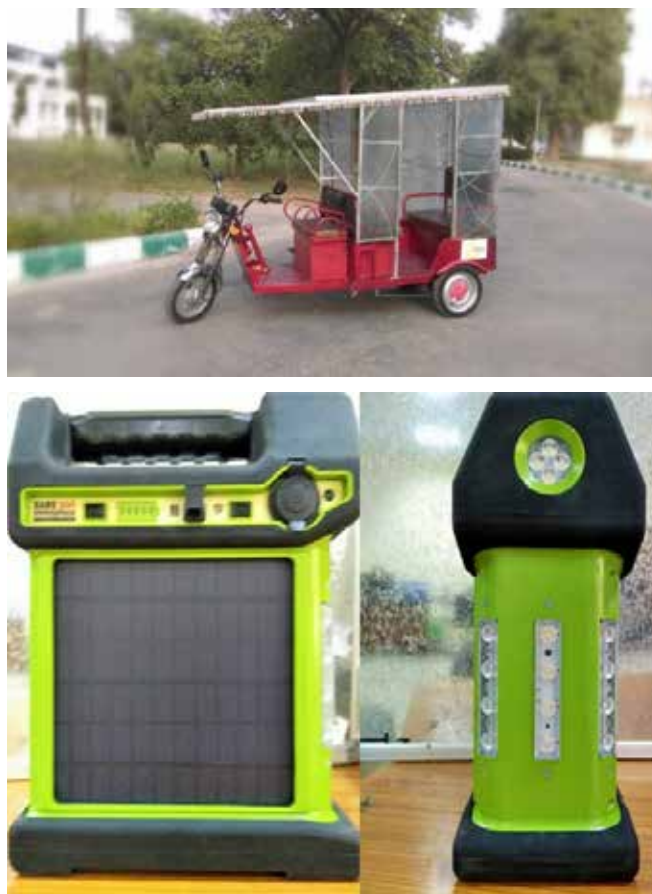
Figure 4.11 : Solar E-rickshaw & User defined solar power pack
