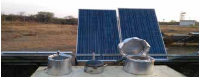
Figure 6.6 : Solar PV based cooking system with thermal battery
