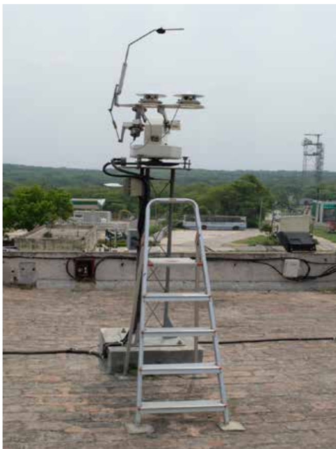
Figure 3.2 : GHI, DHI and DNI Measurement setup
