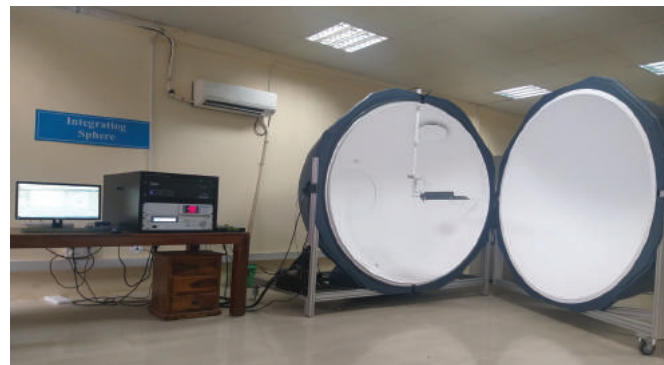
Figure 4.6 Testing of Solar Street Lights and Integrating sphere system with temperature control
