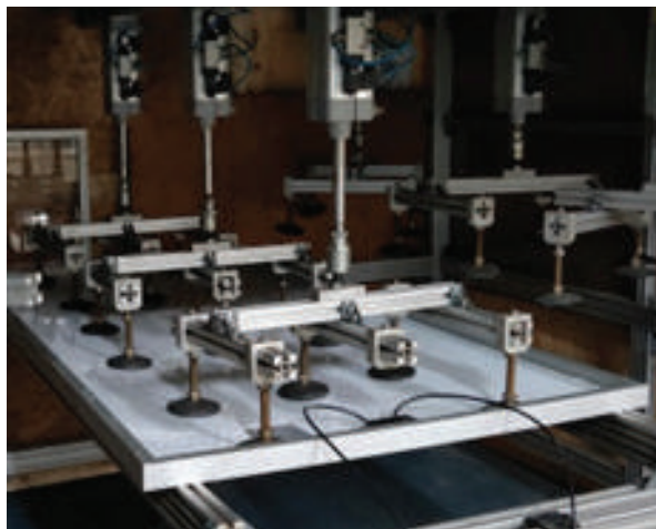
Figure 7.7. Mechanical load tester and EL image of PV module before and after stress
