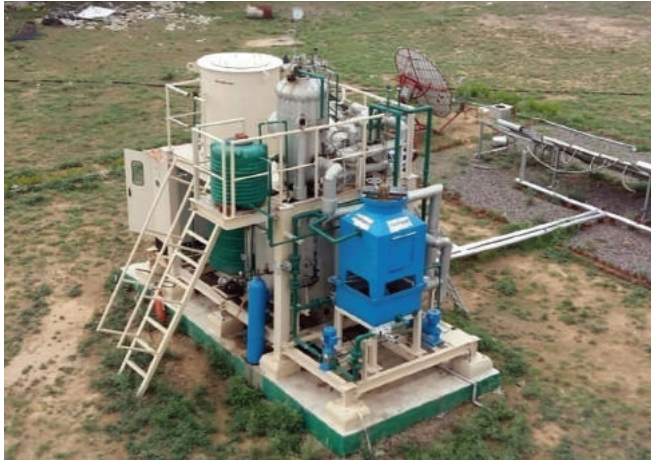
Figure 5.3: Test facility for testing of hot water/steam based CST systems
