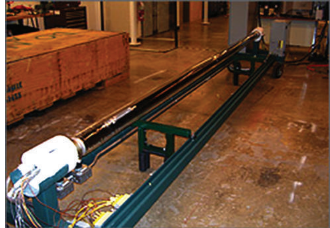
Figure 5.3: Test facility for testing of hot water/steam based CST systems
