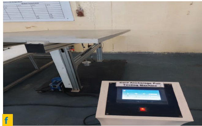
Figure 4.1. Test equipment at Module Testing Lab: (a) EL imaging setup, (b) Heating chamber, (c) Robustness of termination tester, (d) Cut susceptibility tester, (e) Module breakage tester and (f) Chord anchorage tester.
