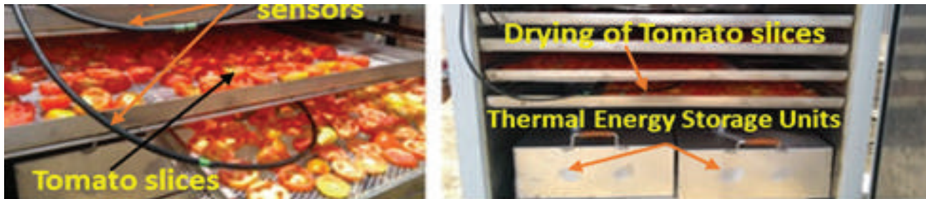
Figure. 7.10 Experimental Testing of Solar Dyer
