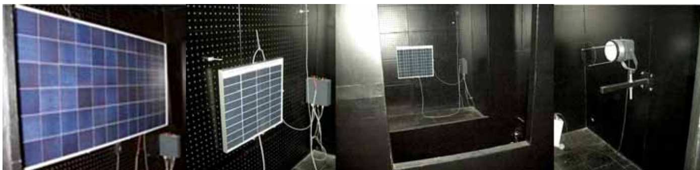
Large area sun simulator quick sun 700A
