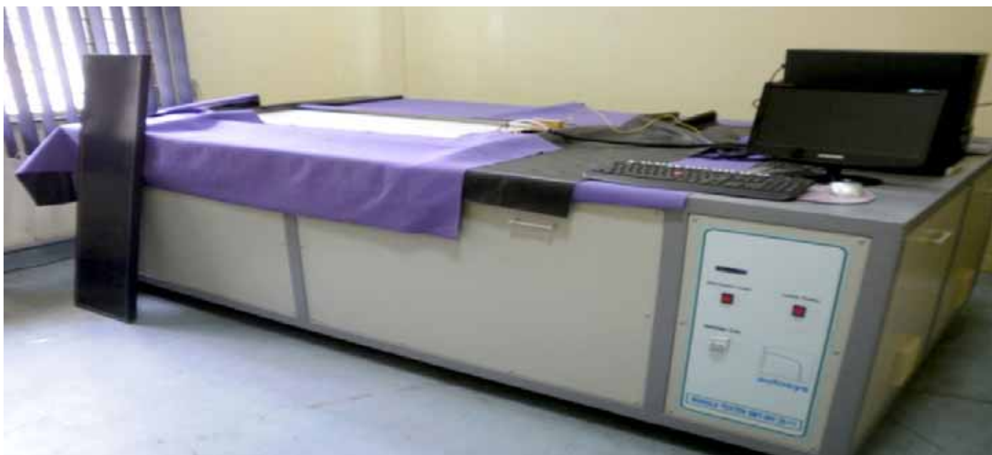
25 kWp crystalline silicon module test bed
