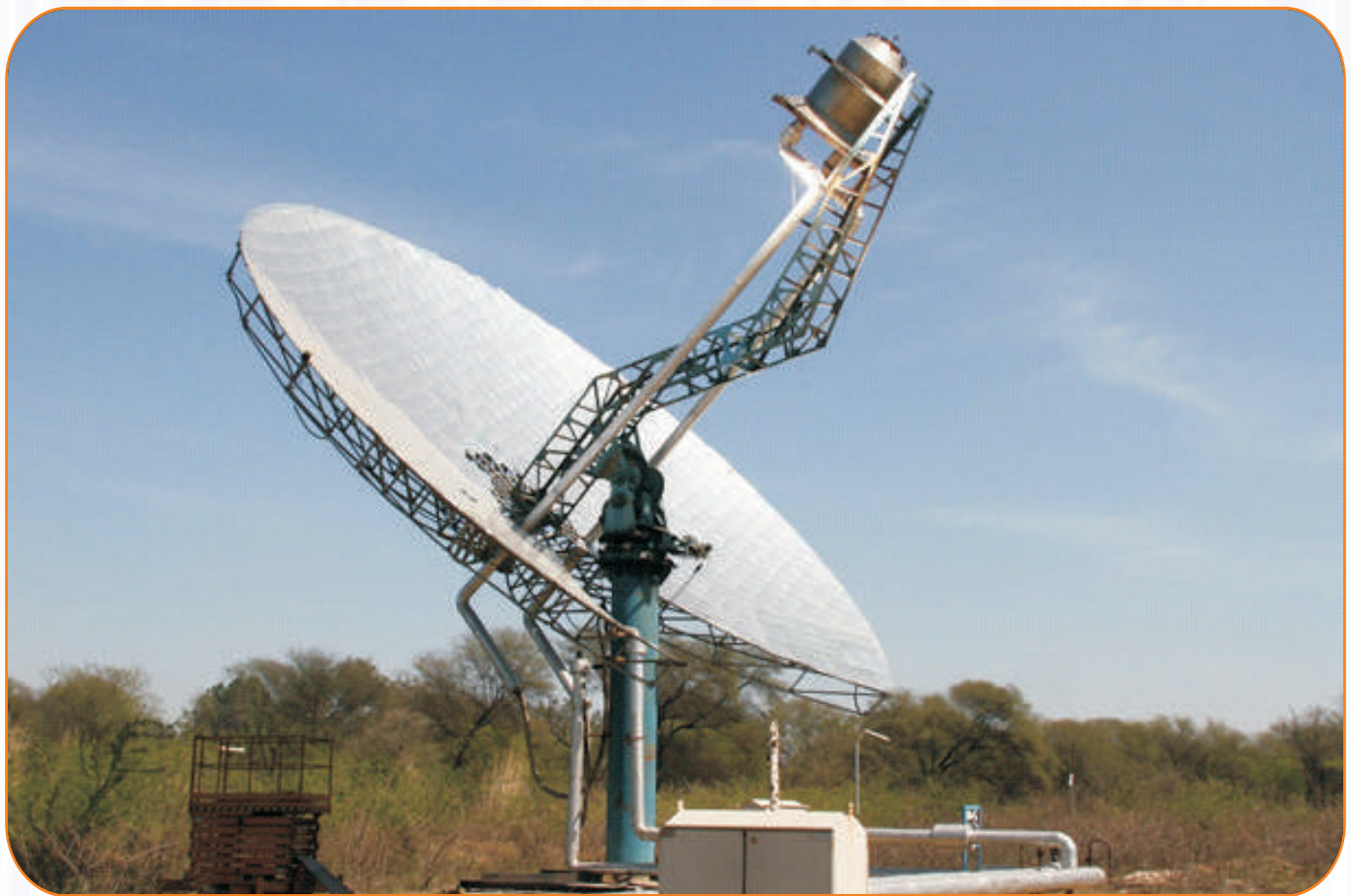
Fig.3.11: Paraboloid Dish for Industrial Process Heat Applications
