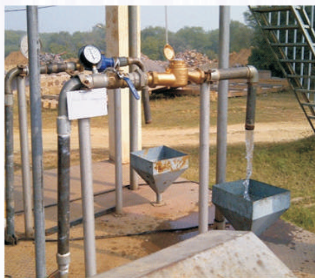
A Solar Water pumping testing Rig.
