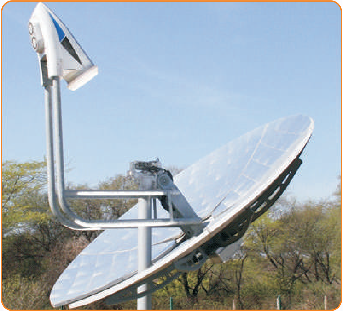
Fig. 3.10: Solar Stirling Engine at NISE
