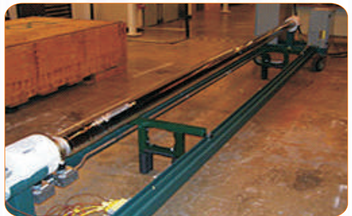
Figure 3.15: Heat loss testing of heat receiver
