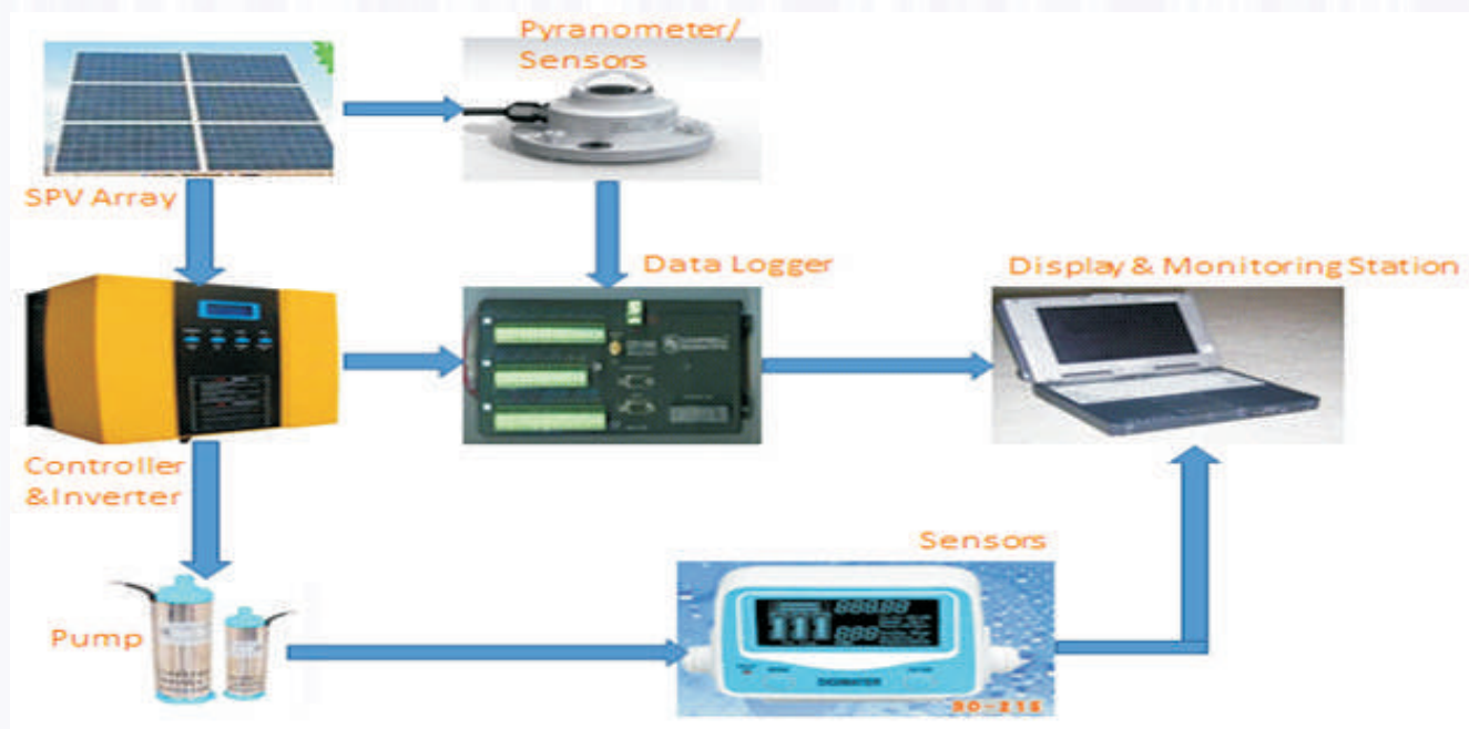
A Schematic diagram of Automatic Solar Water Pump test Set up
