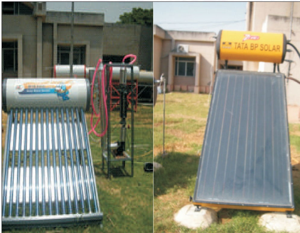
Figure.3.18: Test Setup for solar water heating system
