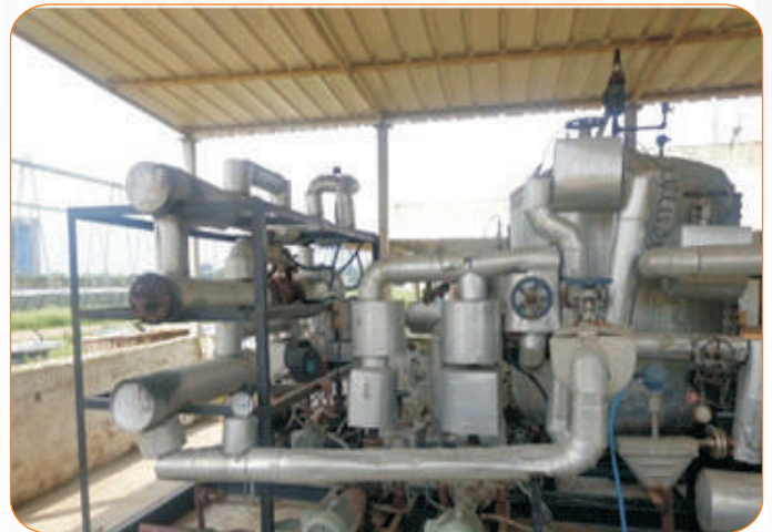
Figure 3.14 : Thermic fluid based Test Set-up for CSTs at NISE
