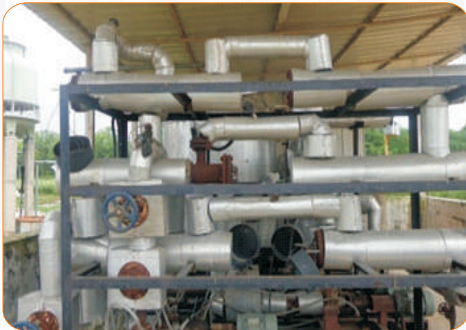
Figure 3.14 : Thermic fluid based Test Set-up for CSTs at NISE
