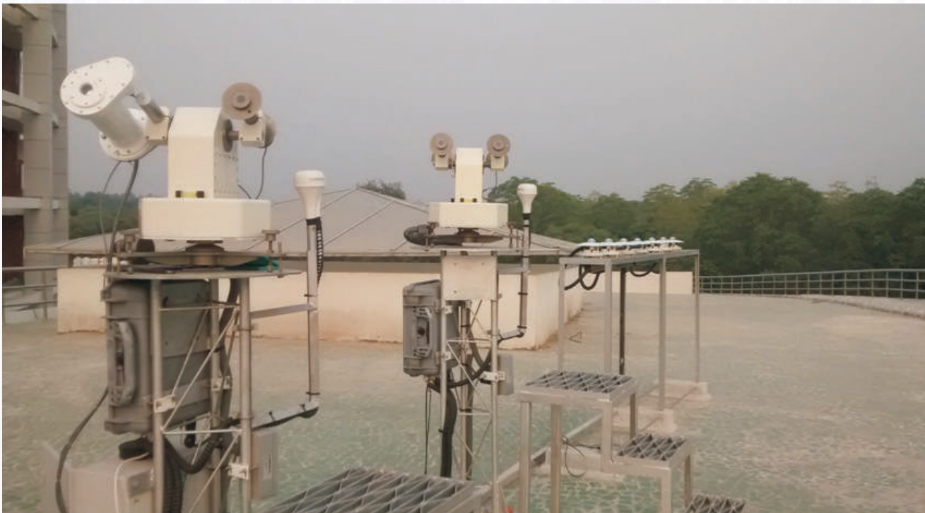
Figure 1.3 Calibration Facility for Solar Radiometers at NISE
