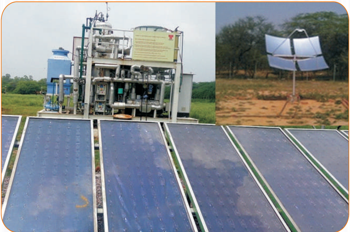
Fig.3.13 : Testing of Evacuated FPC and Solar Dish for High Temperature at NISE
